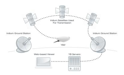
The YB3<sup>i</sup> allows you to track the position of your assets, and send and receive short messages from anywhere on Earth with a clear view of the sky. It can transmit using either GPRS or Iridium satellite, and works far beyond the reach of standard WiFi and GSM networks.
