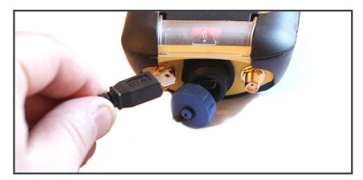
The estimated charging time to fully charge the device is 7 to 8 hours from completely discharged.
