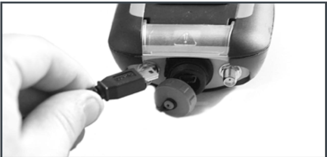
The estimated charging time to fully charge the device is 7 to 8 hours from completely discharged. The device can be used whilst charging, however, the charging cycle will complete more quickly if the device is deactivated. The device can be used with a partially charged battery.
